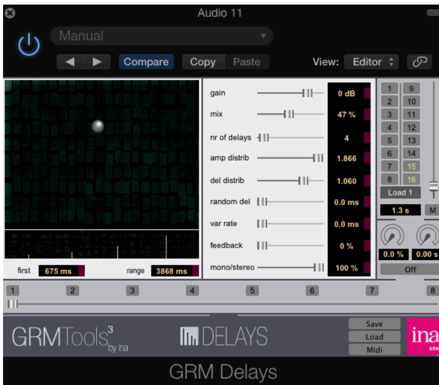
Fig. 12, GRM Tools Delay– using feedback the series of gradually louder delays will repeat
